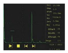
Internal finite echo recording or external infinite USB dynamic recording function to achieve recording full scanning process.
