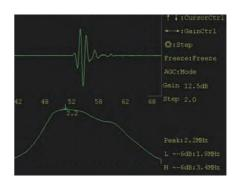
The probe waveform, spectrum and center frequency of the probe can be measured precisely by capturing echoes.
