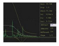
The weld groove profile function can directly point out the location of the defect.
