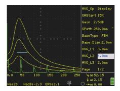
AVG/DGS curve will be auto created by taking a known flat-bottom hole or large flat-bottom echo for reference.
