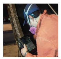
The CTS-9009PLUS is designed to increase productivity in various inspection situations. It is suitable for inspection flaw position and size, which can be widely used for various detection demands, such as pipes and tubes, welding seams, pressure vessels and airplane parts.
