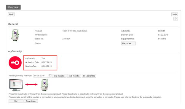
If the instrument is not re-connected on time (or before) to myWorld the instrument gets blocked and cannot be used anymore unless it is connected to myWorld to repeat this procedure to set a new mySecurity renewal date.
