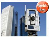
The auto-pointing accuracy with the standard prism is 1" (1 mm at 200 m), and 4" (1 mm at 50 m) with a reflective sheet.
