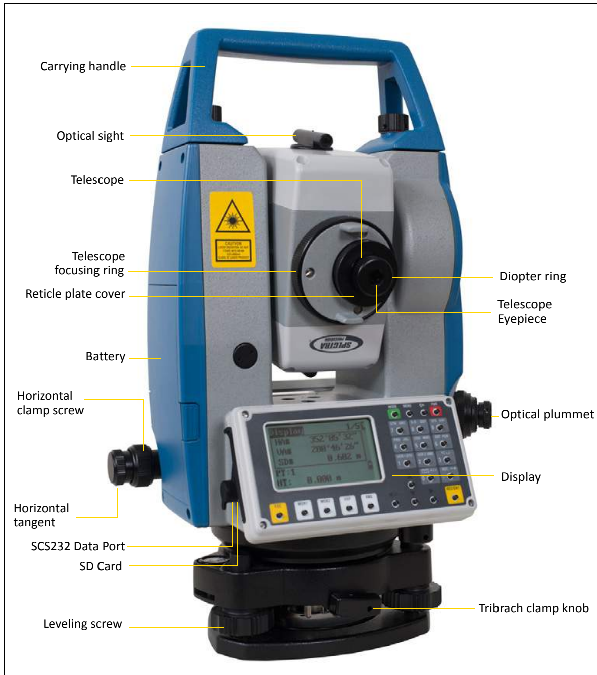
Figure 1.1 FOCUS 2 Series total station: Face 1
