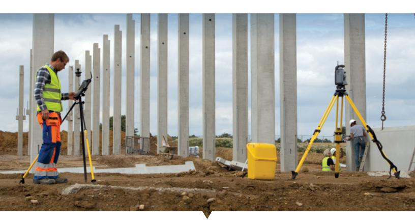
Trimble VISION technology integrates calibrated digital cameras with Trimble S9 and S7 total stations, as well as the Trimble SX10 scanning total station. These instruments have the ability to collect survey data, stream video from the perspective of the instrument, and capture panoramic still images. Trimble Access field software overlays survey data on the streaming video, which enhances your field productivity when operating the instrument robotically.
