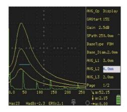
Three curves of different equivalent values will be auto created by taking a known flat-bottom hole or large flat-bottom echo for reference.
