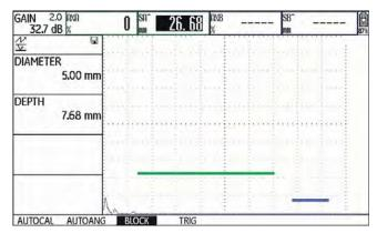
The side-drilled hole is located at a depth of 7.68 mm and has a diameter of 5.00 mm.
