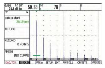
Select the function gate a start and position the gate A on the first DAC echo.
