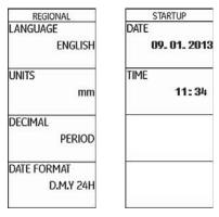
The date is saved together with the inspection results. You can set the date format, the date, and the time using the corresponding functions of the function group **CONFIG1** on the second operating level.
