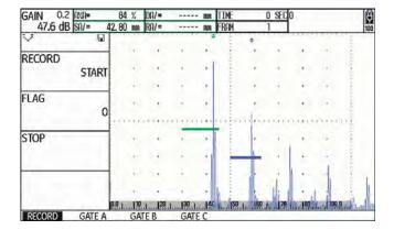
Next to the A-scan, the control functions are displayed in the function group **RECORD**, whereas the settings for each gate in question are displayed in the function groups of gates.
