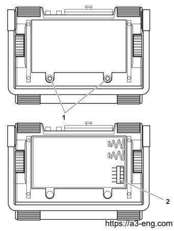
Place the battery in the battery compartment so that the marking faces upwards and the contacts are pushed against the connector pins (2).
