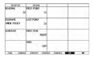
The data recorder enables you to easily manage test tasks with wall thickness measurements, and to store and to document readings in a structured manner with or without an A-scan.
