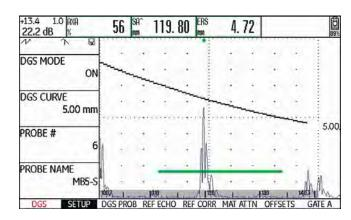
Taking the general DGS diagram as a basis, the USM 36 calculates the required test sensitivity for displaying the 3mm curve with its maximum at 80 % screen height, and makes this setting. The current gain is set to 0 during this.
