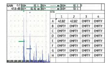
To finish storing the readings, press one of the two selector keys for 3 seconds.
