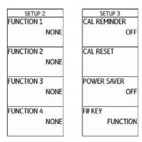
You can assign various functions to the four function keys **F1** to **F4** below the display screen so that you will be able to trigger these functions any time without switching the operating level.
