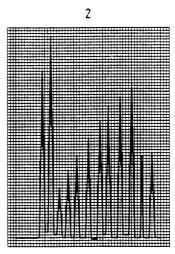
Figure C.1 - Two examples of traces from a discontinuity intensity measuring equipment
